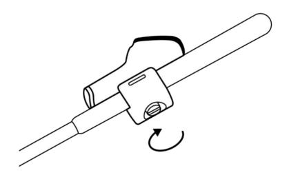
Then, so that your Rango is well attached to your cane, remember to tighten the screw grip with the help of a coin. Check that Rango does not move. If so, Rango is in place.
